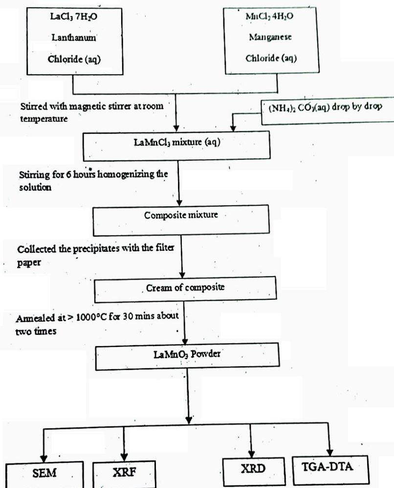
Fig. 1 The block diagram of preparation of LaMnO<sub>3</sub> Powder
